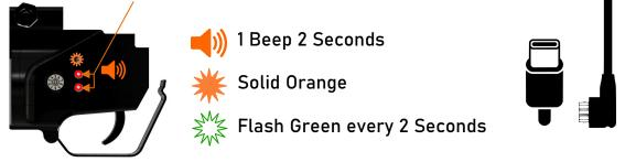
This will validate the unit is correctly receiving a trigger signal without live firing. If a signal is received, the LED will flash orange with a short beep each time a trigger signal is received.
